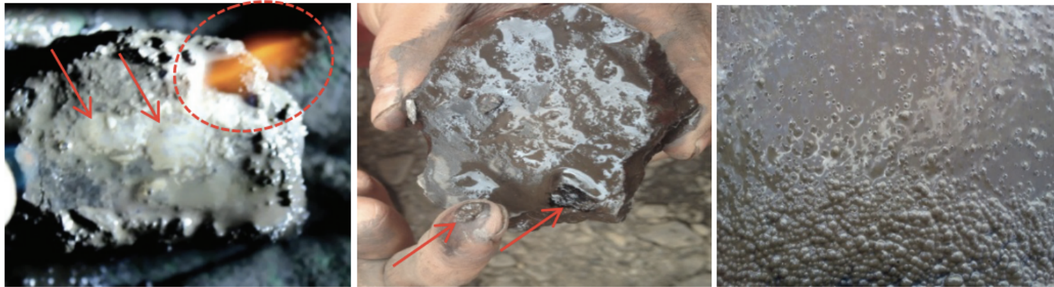
Fig. 3 Abnormal indications within gas hydrate. Note: left-the lump gas hydrate and burning; middle-black heavy hydrocarbon occurs with gas hydrate; right-bubbles of slurry increasing violently near the gas hydrate stratum.
