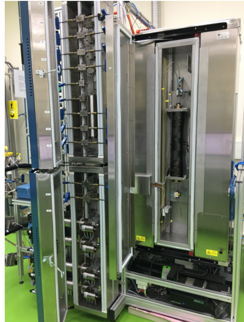
HPHT coreflooding apparatus with X-ray capability
