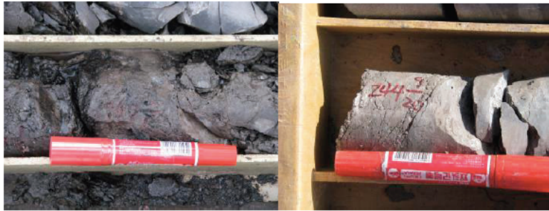
Fig. 3 Example of photos related to faults: mud and breccia in mudstone at the depths of 238.81m (left) and 402.71m (right)
